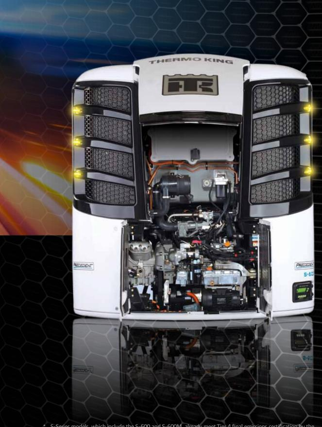
S-Series models, which include the S-600 and S-600M, already meet Tier 4 final emissions certification by the Environmental Protection Agency (EPA) and California Air Resources Board (CARB). Further, they comply with CARB's Ultra-Low-Emission Transport Refrigeration Unit In-Use Performance Standards (ULETRU).
